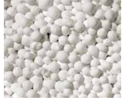
Desiccant Adsorption of water vapour and carbon dioxide. Exhausted during the heat-less regeneration cycle.
