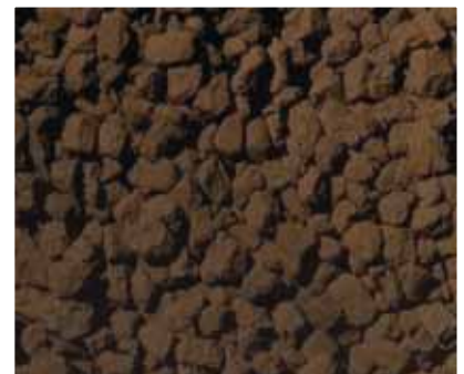
Catalyst A heterogeneous catalytic reaction converts carbon monoxide into carbon dioxide.
