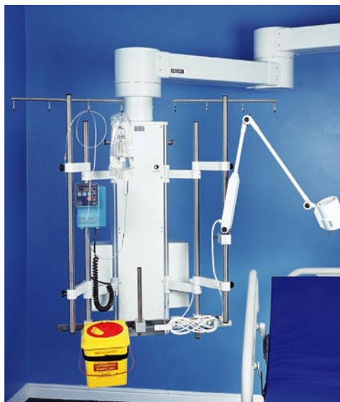
Pendant head configured with examples from the range of accessories. Pole mounted examination light, sharps bin holder, short utility post, cord wrap and coiled lead set (on IV pump)
